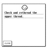
This message is displayed when the upper thread is broken or not threaded correctly, and the "Start/ Stop" button or the "Reverse/ Reinforcement Stitch" button is pressed
